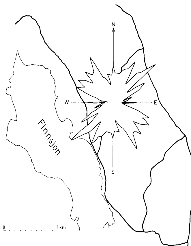
Figure 4-4. Diagram showing the direction of 448 steep fractures within the study area at Finnsjö Lake. The fractures are irregularly oriented in widely varying directions. (Bedrock Bureau, Geological Survey of Sweden).
